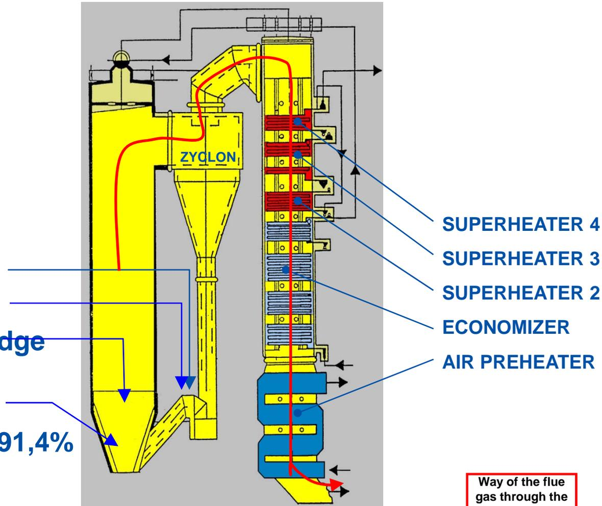
Way of the flue gas through the boiler
